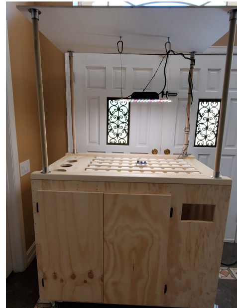
Fig. 7. The overall build of the Automated Home Hydroponics System provides a solid addition to any indoor space. Structure Dimensions: 4' X 29.5" X 6.5' (L x W x H)
