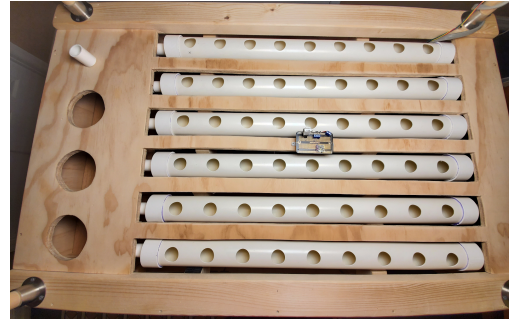
Fig. 6. The essential PVC construction atop the cabinet of the Automated Home Hydroponics System that houses the plants and provides a path for water to flow to them.
